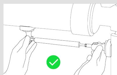
Do not grab the shaft to remove sensor. Only remove by grabbing the end joints.
