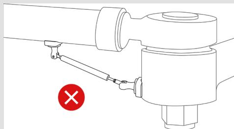
The sensor should be in the centre of its movement. (Showing close to 25mm on the MultiTool Pro).
